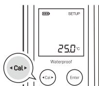
5. Press the **Enter** key to save and press the **Meas** key to return to the measurement mode.
