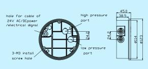
Note: the diagram is for cast aluminum housing
