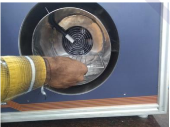
STEP – 8 : Replace the inner chamber & grill plate
