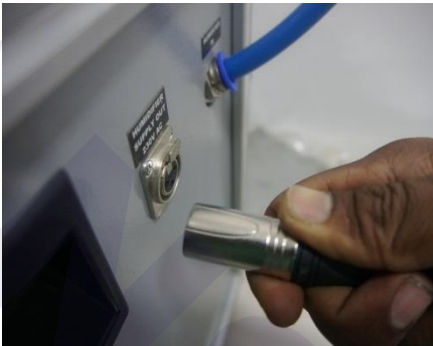
STEP - 2 : Remove the HCAL 1104U side humidifier supply Out connector as above image
