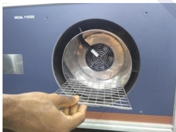
STEP – 4 : Remove the Inner grill plate
