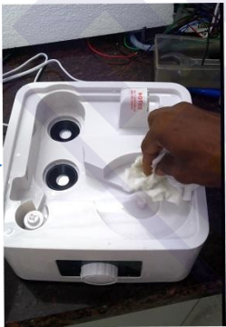
STEP - 3: Remove the Humidifier tank (Refer. 3.5.), drain the water and dry the humidifier area carefully as per above image.
