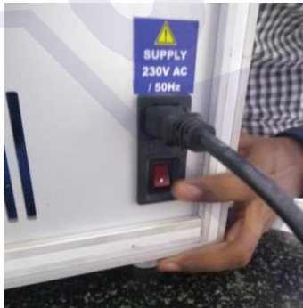
STEP - 1 : After completion of calibration, Switch OFF the HCAL 1104U.
