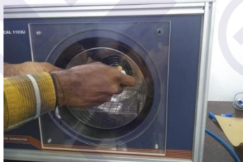
STEP – 9 : Replace the Front acrylic door and close using 4 knobs
