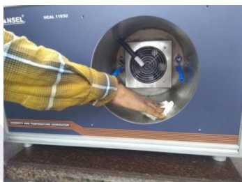
STEP – 6 : Clean chamber surface thoroughly using tissue paper
