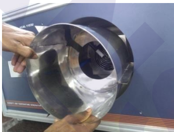
STEP – 5 : Remove the Inner Chamber
