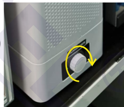
Switch ON this knob during above Ambient Humidity set value (Example : If ambient Humidity value = 50%RH, then from 51 to 95%RH)
