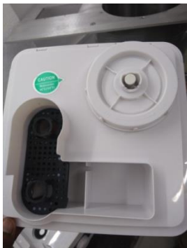
STEP - 3 : Place the Tank upside down and open the cover by rotating it anticlockwise.
