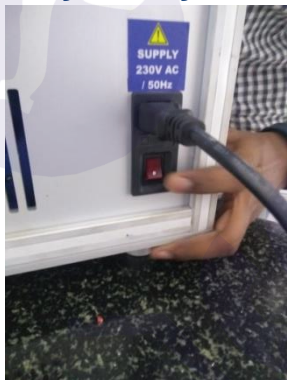
STEP – 1 : Switch OFF the HCAL 1104U
