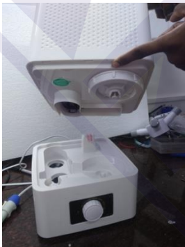
STEP - 2 : Carefully lift the Humidifier tank.
