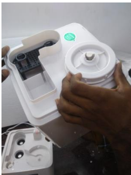
STEP - 3 : Place the Tank upside down and open the cover by rotating it anticlockwise.
