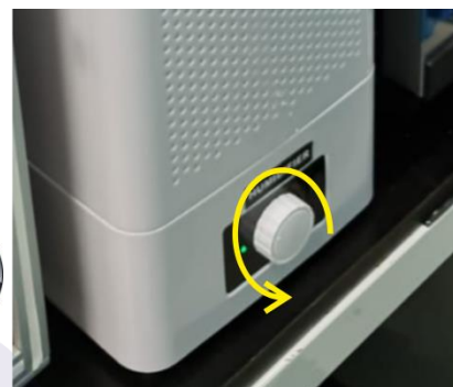
Switch OFF this knob during below Ambient Humidity set value (Example : If ambient Humidity value = 50%RH, then from 10 to 50%RH)
