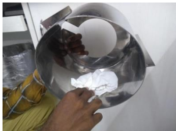
STEP – 7 : Clean inner chamber thoroughly using tissue paper
