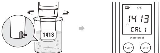
3. Press the **Enter** key, the default calibration value begins flashing.
