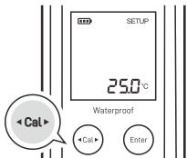
4. Place the electrode into a solution with a known accurate temperature and wait for the measurement to stabilize.
