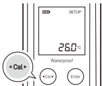
6. Press the **Enter** key to save and press the **Meas** key to return to the measurement mode.
